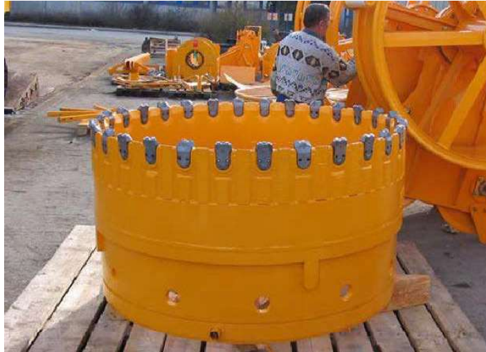
Figure 5-14 Cutting Shoe for Segmental Casing
