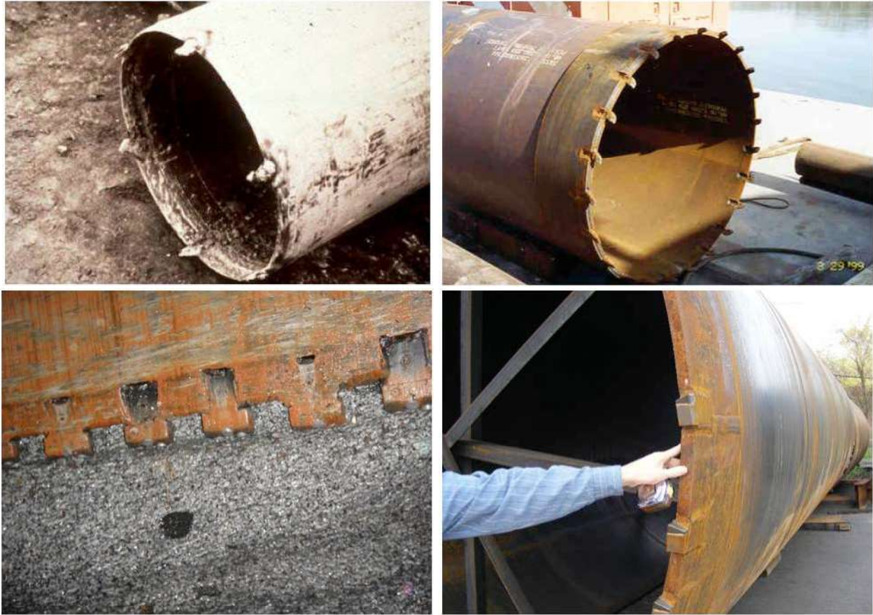
Figure 5-8 Teeth for Use in Sealing Casing into Rock (Photograph at top left courtesy of Herzog Foundation Drilling, Inc.)
