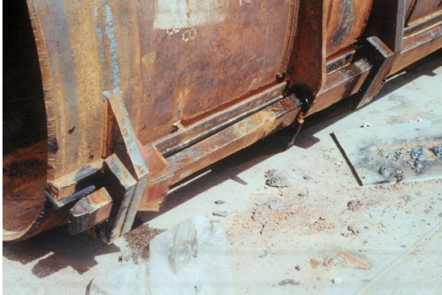
Figure 5-17 Locking Mechanism for a Removable Casing
